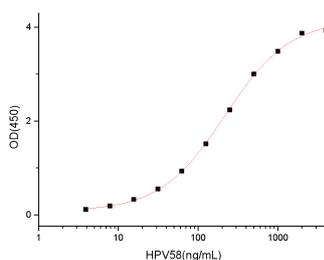
Four-parameter fitting standard curve (linear correlation coefficient  $R^2=0.99943$ )
